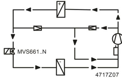
Suction pressure and temperature are monitored with a mechanical capacity controller and reinjection valve.
