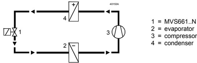
Electronic superheat control is achieved by using additional control equipment (e.g. PolyCool).
