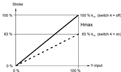
When  $k_{vs}$  reduction (DIL switch 4 in position ON) the stroke will be limited to 63 % mechanical stroke. 63 % of full stroke then corresponds to an input / output signal of 10 V. If, in addition, the stroke is limited to 80 %, for example, the minimum stroke will be  $0.63 \times 0.8 = 0.50$  of full stroke.
