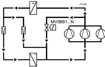
Suitable for large refrigeration systems on air conditioning applications with several compressors or compressor stages, and where the evaporator and compressor are some distance apart (attention must be paid to the oil return).
