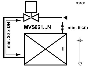
Laboratory measurements reveal that control performance improves when the refrigerant valve is installed so that it is higher than the evaporator (min. 50 mm).
